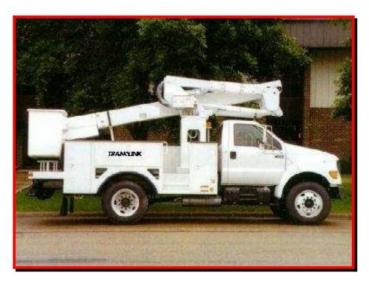
The RANGER RTI Series is mountable onto a wide range of chassis types to suit all applications. It is available with a single or two person platforms and as a material handling device with winch and jib (454kg capacity) (except RTI-110).
